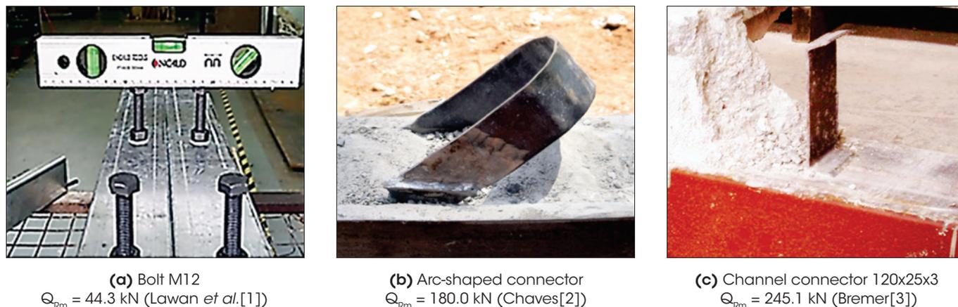
**Figure 1** Shear connectors suggested for CFS composite beams and their average strength
