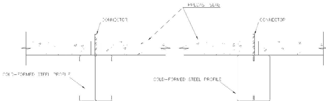
**Figure 2** Steel plate with holes applied to CFS composite beams in precast floor systems
