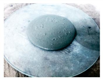
Figure 4 Slump-flow of mortar with 0.30 for f/c and 0.40% for sp/c
