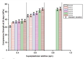
Figure 7 Compressive strength at 28 days for self-compacting mortars
